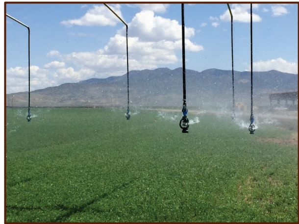
Nozzle upgrades on Farm and Ranch center pivots Source: Ute Mountain Ute Tribe
